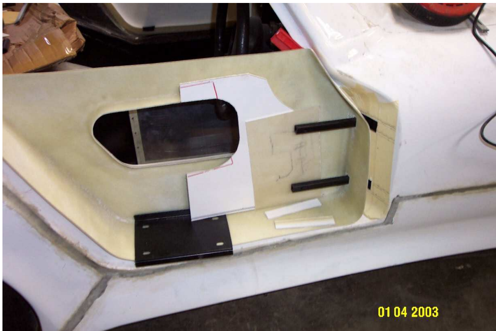
Packing door hinge to inner skin
