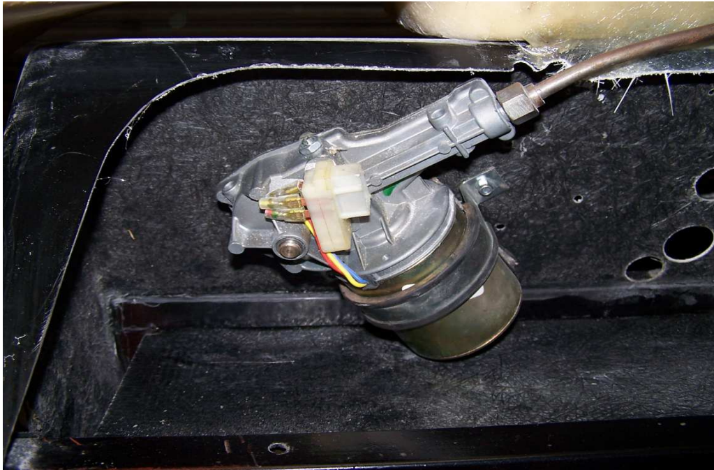
Keep the bottom of the wiper motor above the chassis cross member The motor is located through the bulkhead,
