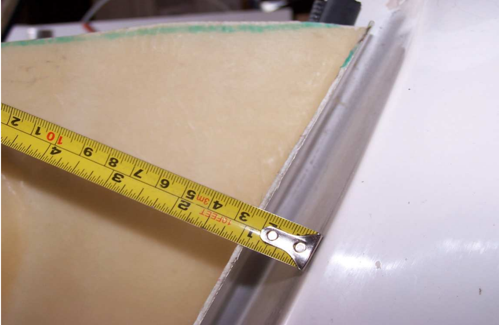
The gap at the back of the door between inner door skin and body shell About 20mm. (Its not the same all the way down)
