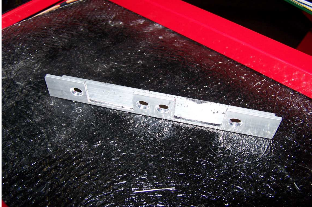
Alloy bracket for fitting fuse box to.
