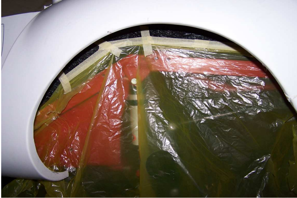
Cover up chassis before fibreglassing. Do the same at the front end
