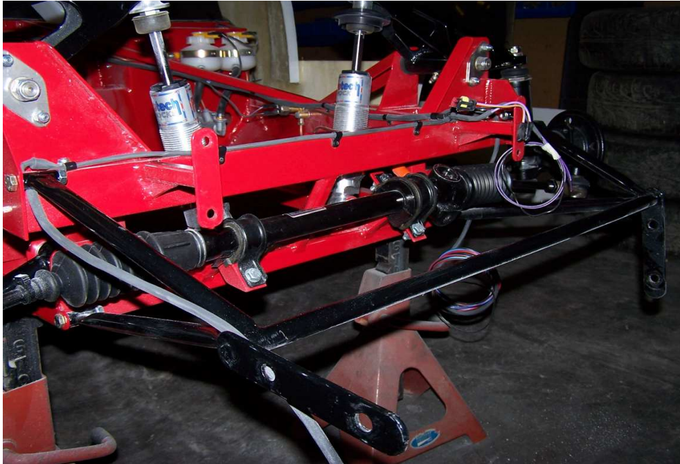
Steering rack in position on a LHD car
